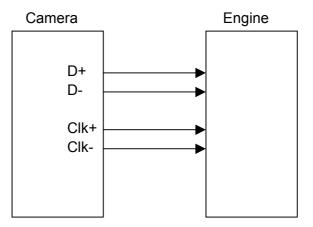
D+ and D- are differential picture data output from the camera module. This data is written on each falling edge of **Clk**. Data format is least significant bit first. When nothing is being transferred, **D** remains high, except in power shut-down.
