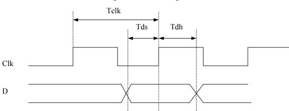
Figure 3: Basic bus timing
