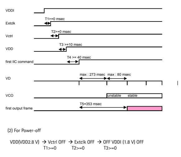
Figure 9. operation sequence in power-on
