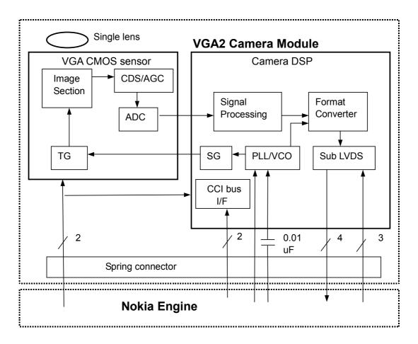
Figure 1: Block diagram of camera module
